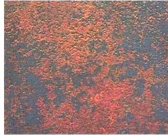
Condition B Unblasted
